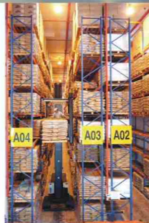
Very Narrow Aisle Rack Configuration
