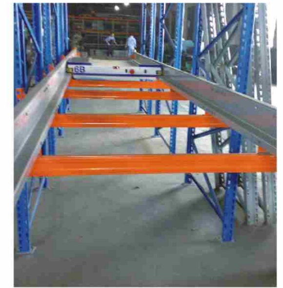
Shuttle car can move the shelves from the depth of the tray to the front, use the forklift to take down the goods. 穿梭车将货物深处的托盘移动至货架最前端，用叉车将托盘货架从上取下。
